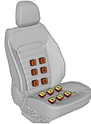
Figure 2-39 Configuration of sensor arrays on the passenger seat
